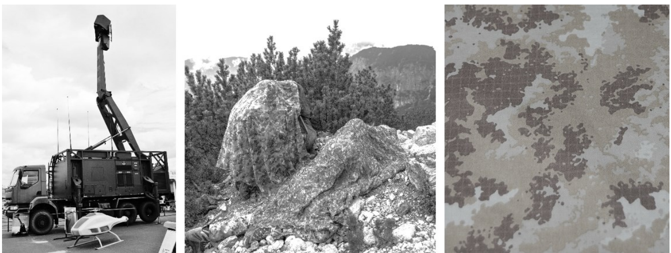
Fig. 44 A Saab-Ericsson Giraffe AMB radar displayed at the Paris Air Show, 2007. Originating from Sweden and introduced in 1977, this early warning radar operates in the C band, S Band, and X band frequencies. With around 450 units built, it boasts a rotation per minute (RPM) of 60, a range between 10 and 470 kilometres, and can detect altitudes between 0 and 40,000 metres, specifications varying by variant. Photo by: Duch.seb. Date: 24 June 2007. Credits: Attribution-ShareAlike 3.0 Unported (CC BY-SA 3.0). [File: Giraffe AFB-radar.jpg]. Source: wikipedia.org. Fig. 45. An Italian Special Forces Sniper team anticipates their target during a STALK exercise at the International Specialty
